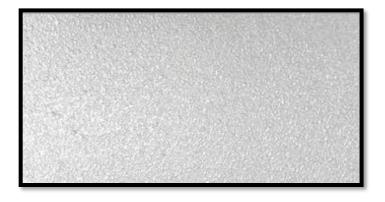
Apply 2 - 3 uniform layers with an anti-gravel gun at an average pressure of 3.5 - 4 bars, at a distance of 30 - 40 cm from the surface. Wait for 20 - 40 minutes and apply 1 effect layer with an anti-gravel gun at an average pressure of 3.5 - 4 bars, at a distance of 30 cm from the surface.
