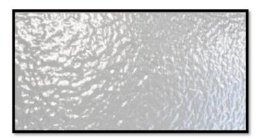
Apply 2 wet layers with an anti-gravel gun at a medium pressure of 2.5 - 3 bars, at a distance of 20 - 30 cm from the surface.
