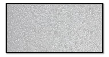
Apply 1 - 2 wet layers from an anti-gravel gun at a medium pressure of 2.5 - 3 bars at a distance of 20 - 30 cm from the surface. Mix PROTECTIVE COATING with hardener. Wait for 20 - 30 minutes and apply 1 uniform layer with an anti-gravel gun at low pressure 1.5 -2 bars, distance from the surface: 30 - 40 cm
