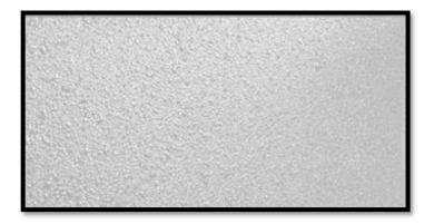
Apply 1 - 2 wet layers from an anti-gravel gun at a medium pressure of 2.5 - 3 bars at a distance of 20 - 30 cm from the surface. Wait for 20 - 40 minutes and apply 1 - 2 effect layers from an anti-gravel gun at a medium pressure of 3 - 4 bars, distance from surface: 40 – 50 cm
